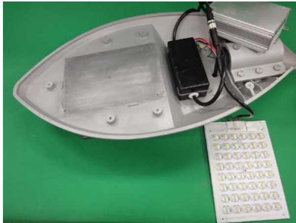
Fig. 4. Streetlight as received by LED North America showing the location of the LED board on the aluminum housing
